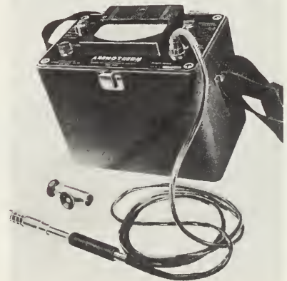
23-23. A direct reading air velocity indicating instrument. (Anemostat Corp. of America)
